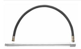
Suction assemblies for wall mounted stub pumps, drums and tanks. Assemblies include  $\varnothing$  42 suction tube with foot valve, height adjustable 2" bung adaptor and 2 m x 3/4" rubber connection hose. 1060 mm suction tube.
