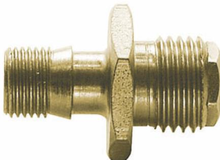
Pressure relief valve, 1/8" BSP (M) - 60 bar approx. opening pressure. When mounted to the pump body, prevents damage in the system caused by over pressure produced by thermal expansion (1 °C increase in temperature can cause up to 10 bar increase in the system pressure). Opens at approx. 60 bar. Possibility to connect either a 1/4" hose with a clamp or a hose with 1/8" BSP (F) fitting as oil return line.
