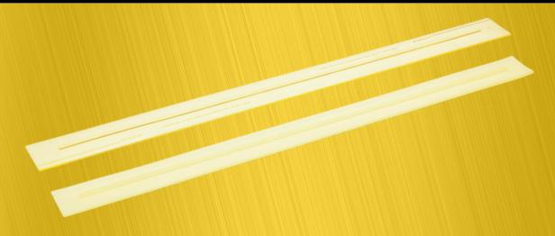
The suction lip set consists of a front and rear suction lip. The length is 890 mm. The suction lips are closed and are made from high-quality, oil-resistant and transparent polyurethane with a long life. Suitable for textured floors.
