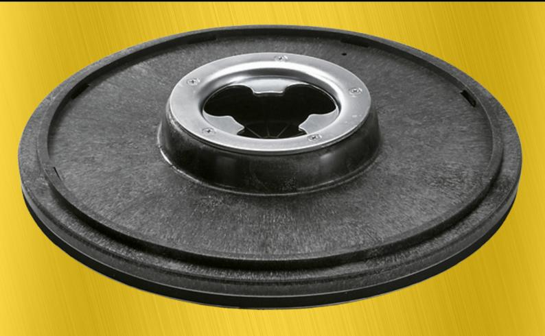
Pad driver plate (low-speed) for cleaning with pads using machines up to 200 rpm. 420 mm diameter. Pad driver plate features a quick-change coupling and centre lock.
