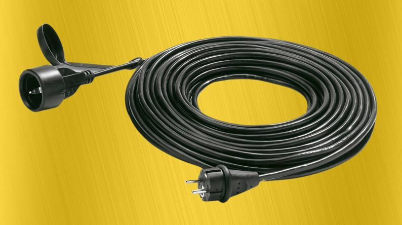
Extension cable (20 m, 3x1.5 mm²) with splash-proof earthing pin plug, strain relief and anti-kink sleeve.
