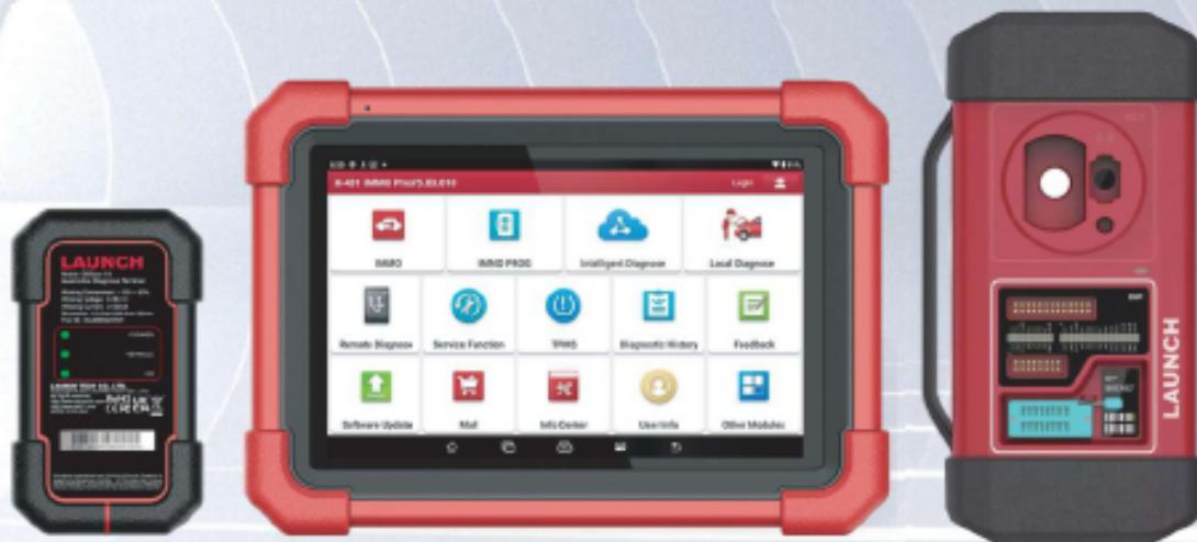
X-431 IMMO PRO is a latest new product line scan tool from the Key & IMMO Programmer family for car security and immobilizer systems, featuring complete IMMO & Programming services and intelligent diagnostics (basic diagnostic functions included).
