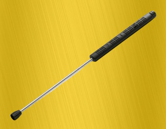
For all high-pressure cleaners in the Classic range from Kärcher: 850 mm long, galvanised, non-rotatable spray lance. Can be used at water temperatures of up to 60 °C and working pressures of up to 250 bar. With manual screw fitting, M 22 × 1.5 thread for connection to the high-pressure gun, as well as M 18 × 1.5 thread for connection of accessories.
