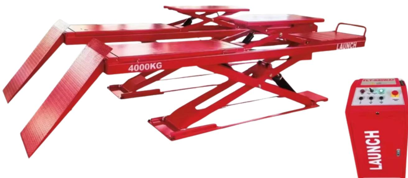
The TLT840WAF Big Scissor Lift takes space-saving style to save most workspace for diagnostic business. The rated load reaches 4000kg. Many physical installations and settings ensure effective and efficient operations to be safe and reliable. It has very good horizontal adjustment ability for precisely adjusting horizontal accuracy for the four-wheel alignment detection.
